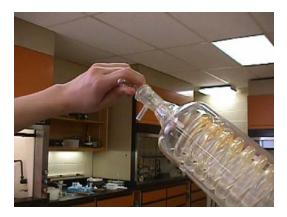
4. The flask should then be rotated by turning on the appropriate dial. Since evaporation cools down the pot, it is then immersed in a thermostated warm water bath. This keeps the solvent evaporating steadily. The green light indicates the heating coils are activated. The orange light signals that the bath is heating the water. This orange light goes off when the water temperature reaches the selected value. The temperature selection dial is located at the lower right on the water bath.
