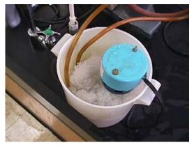
3. Next, the aspirator water should be turned on full force. Then the condenser stopcock is turned at a 90 degree angle to the glass tube in the stopcock to instate the vacuum. The system is now "closed". The aspirator lowers the pressure throughout the apparatus. The solvent in the pot will start to evaporate.
