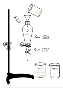
Transfer the entire reaction mixture (using a funnel) to a 125ml separatory funnel (Be sure the stopcock is in the closed position). Two layers should appear. The top layer is the ether layer, containing product. The bottom layer is the aqueous layer containing the magnesium bromide salt by-product. Label two 100ml beakers or Erlenmeyer flasks as "water layer" and "ether layer". Drain the lower layer from the separatory funnel into the beaker or flask labeled "water layer".
